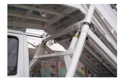
Hydraulic system is constituted of oil cylinder, oil filter, globe valve, oil pump, hand pump, check valve, solenoid directional valve, hydraulic control double check valve, hoist oil cylinder, micro-adjusting oil cylinder, front and rear supporting foot oil cylinder, expansion oil cylinder of platform and unlocking oil cylinder, pressure gauge, oil tube and piping accessories.
