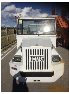
ENGINE: Diesel Deutz F4L912 model aircooled. 4 cylinders. Diameter/path: 100/120 mm. Charge: 3770 litres. Relation of compression: 18. Max. power: 54 KW/2500 r.p.m. Torque engine
