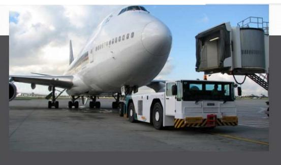
The Flagship F1-500 Aircraft Tractor was designed in Australia for both pushback and extended towing of aircraft up to 600 Tonnes (A380-800). Drop-in ballast in the F1-500 easily transforms the tractor from a standard 54 Tonnes for A340 & B747 up to 70 Tonnes for A380-800 with no obstruction to the operators' line-of-sight.
